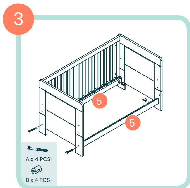
Assemble the two mattress support rails (5) using 4 x A bolts and 4 x B nuts
