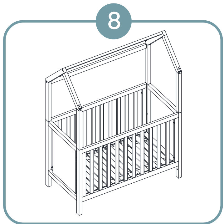
Assemble rail using 6 x A bolts and 2 x H wooden dowels
