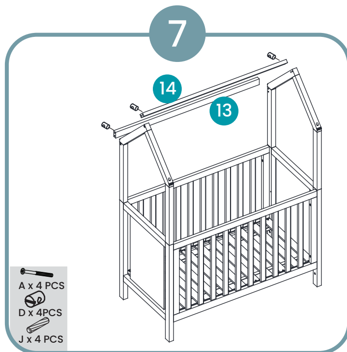
Assemble rail using 4 x A bolts and 4 x D nuts and 4 x J wooden dowels
