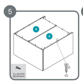
Assemble back using 20 x D screws
