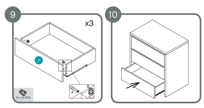
Assemble drawer front to drawer frame using 12 x B locking nuts.
