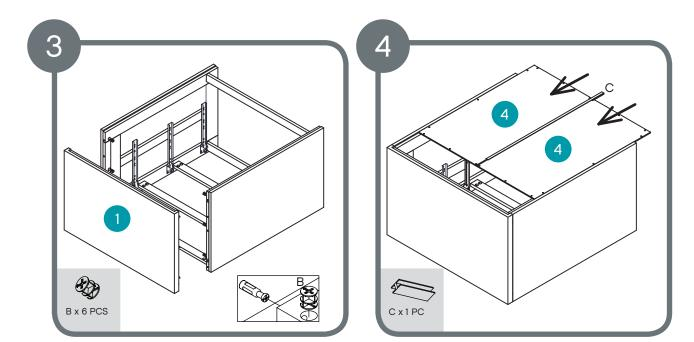
Assemble top to frame using 6 x B locking nuts
