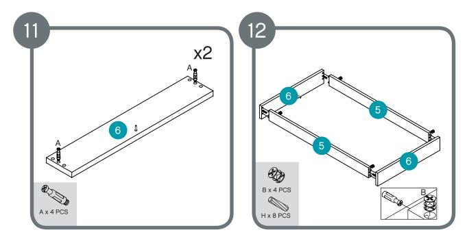
Screw metal pins into short top support bars
