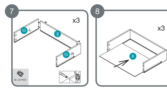
Assemble two drawer sides to drawer back using 12 x B locking nuts Slide drawer bottom into the grooves
