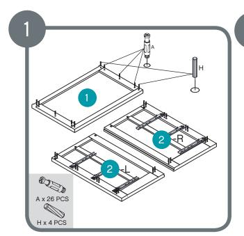
Screw metal pins into top and side Put wooden dowels into top
