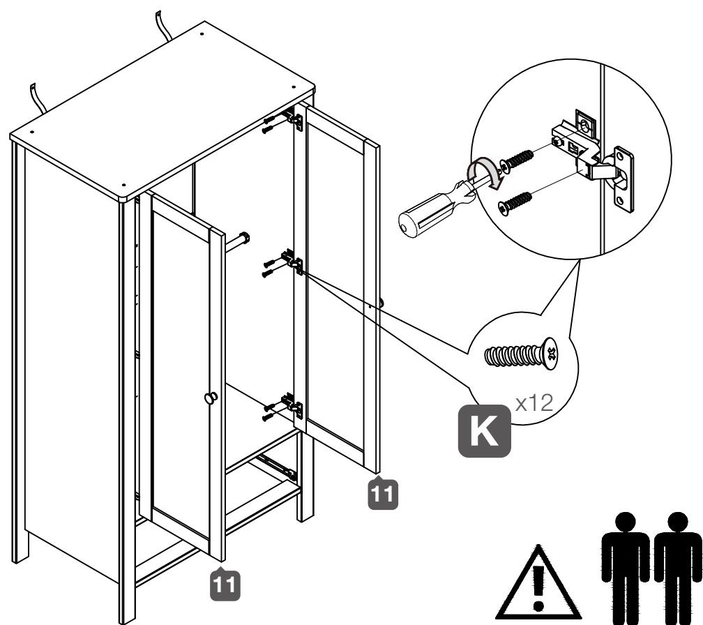
**Adjusting the doors Ajuste de las puertas****Ajustement des portes****Justage der Türen****Registrazione dei portelli****De deuren verstellen****1**
